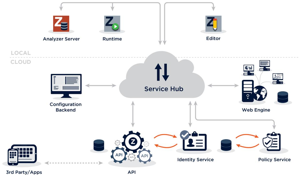
Figure 1: All components in the zenon Service Grid are connected via the central Service Hub. This also constitutes the connection between the local level and the cloud.
