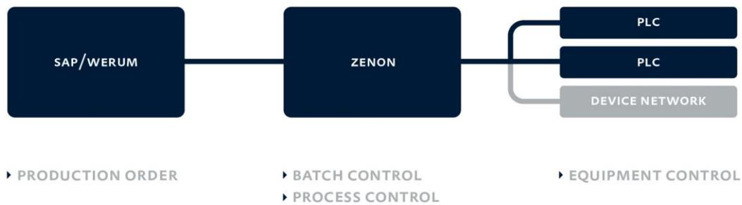
zenon provides the translation from a supply chain production order in the business IT, to control each required process on the OT system. zenon receives the production order through the defined ERP or MES connection, maps these to a Master Recipe, creates a Control Recipe, and when requested starts the production execution. Production status and key values are communicated back up from the equipment to the ERP or MES.
