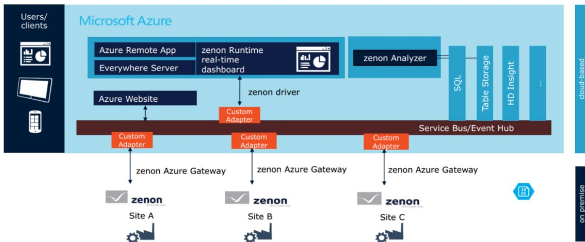
The Azure cloud technology integration into zenon is highly scalable in scope and functionality, effectively extending the zenon structure. For example, historian data can be moved to the cloud enabling efficient data management, storage and analysis; live processes can be communicated opening the possibility of global visibility; with the zenon Analyzer being available as a cloud solution.
