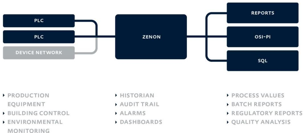
zenon uses its communication library to connect to all production equipment and devices, variables are defined in an alarm structure, and in a historian structure. Using either the Report Viewer or zenon Analyzer, reports can be generated automatically or manually, and stored on a secure server.
