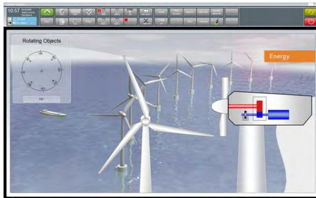
zenon Operator offers all HMI functions that are required in a wind turbine, such as communication to the PLC, display of the current status, archiving of events and alarms and on-site operation of the turbines.
