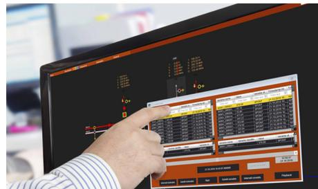
The Process Recorder records data in zenon Service Engine so the data can then be played back later in project simulation mode. This allows problems to be analyzed in more detail after the event (in a Post-Mortem Analysis). This functionality means the Process Recorder can provide a convenient method of performing simulations and training for new employees.
