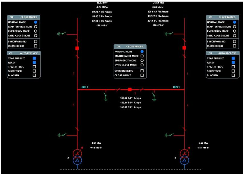
Powerlink’s first in-house developed, designed, tested, and commissioned IEC 61850 station bus solution.
