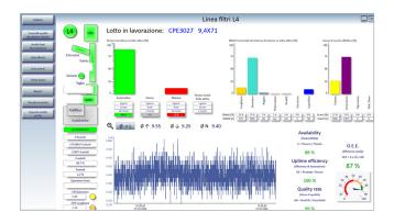
Precise and detailed control of the line, with dynamic colors, dashboards and graphics that clearly show the status of the line, the availability and efficiency of production, as well as the defects and causes of rejects.
